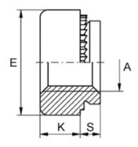
Female thread A = M2Height K = 2.0Max recess height = 1.0Min distance to edge = 3.0Outer diameter E = 6.0Plate thickness = 1.1 to 1.4
